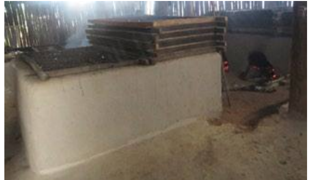
Fish Smoking Oven constructed with Hydroform blocks
