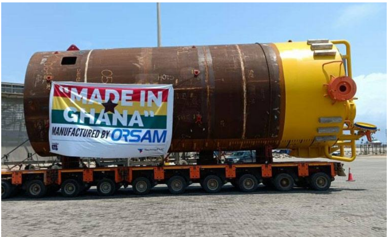
A Riser Pile (60T) fabricated by Orsam as part of the JSE Project.
